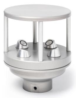
The ultrasonic wind sensor SUW1AE manufactured by PM Ecology has been designed for constant use communications protocol used in harsh weather conditions. The corrosion resistant anodized aluminum housing and no moving parts design, make the sensor ideal for long-term measurements with no maintenance required. Good performance in high winds as well as short response the sensor and the third one transmits the data. time to slight air movements provides accurate
